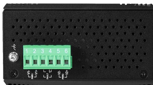
Figure 2.3: Top Panel View of PG5-0602-SFP series
