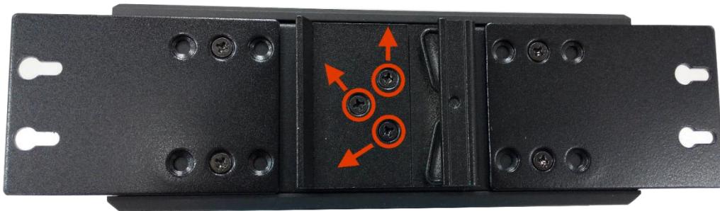
Figure 3.4: Remove DIN-Rail Bracket from the Switch
