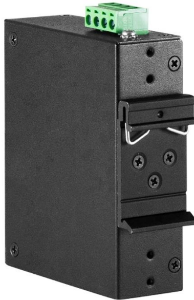
Figure 3.1: The Rear Side of the Media Converter and DIN-Rail Bracket
