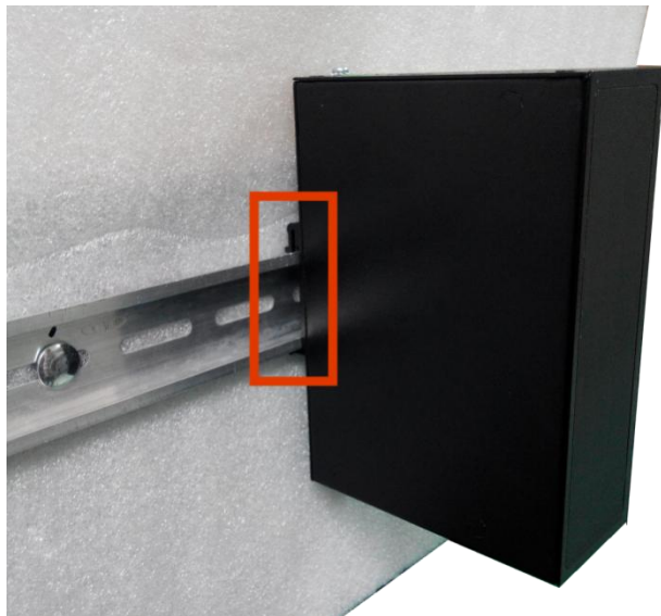
Figure 3.3: Stable the Switch on DIN-Rail
